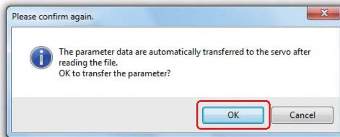
3. Display the setup data on the parameter setup screen and automatically transfer its contents to the servo by selecting the save location at the data save dialog box and clicking "Open".
