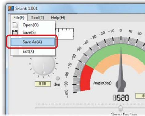
2. When creating a new file with "Save as" since a data save dialog box opens, select the save location and save the setup data of the parameters setup screen to the computer as a file by clicking "Save".
