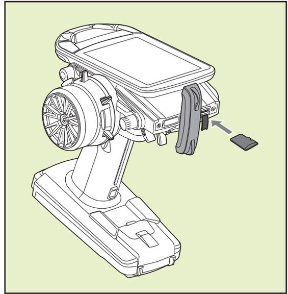
5. Turn on the transmitter power while pressing down the "HOME" button. The update screen appears on the LCD display of your T10PX and the software update is started.
