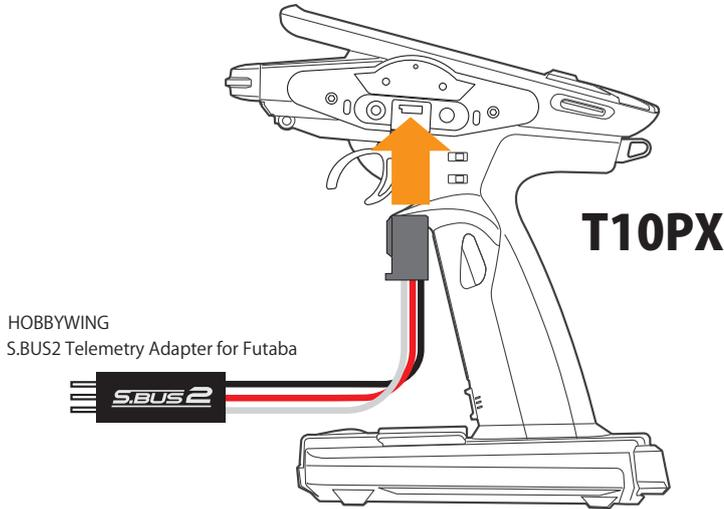
Connect the Hobbywing S.BUS2 Telemetry Adapter for Futaba to the COM port on the back of the T10PX.
