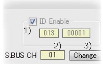
When connecting multiple servos to the CIU-2/3 tick the "ID Enable" check box, input the ID No. of the ID seal attached to the servo whose parameters are to be read, and click the "Connect" button or select "Connect" from the "Tool" menu. If the ID is a mismatch, the Error message shown below (right side) will be displayed and communication will not be established.
