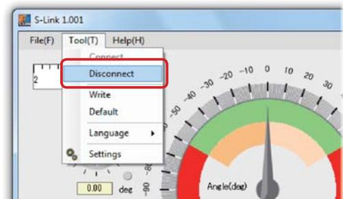
Note: Do not pull out the lead wire or turn off the power while parameters are being written.
