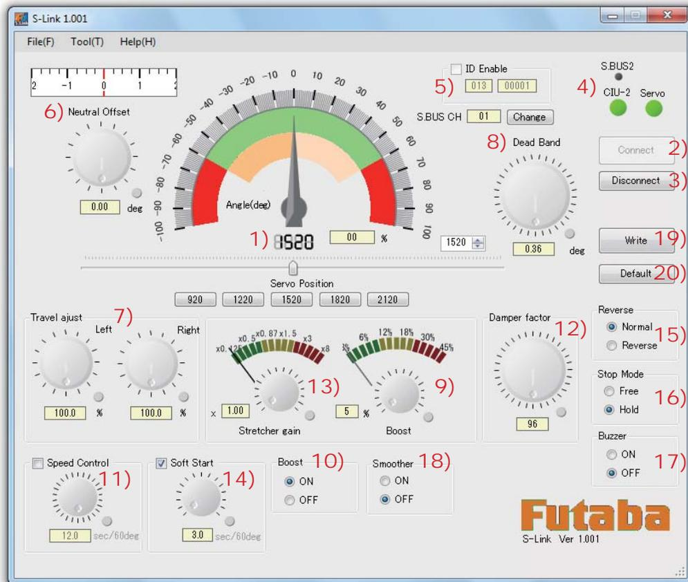
Set values can be changed by clicking or dragging the dial and lever of each parameter. In addition, after a dial or level is selected by clicking, operation by mouse wheel and keyboard arrow keys is also possible.
