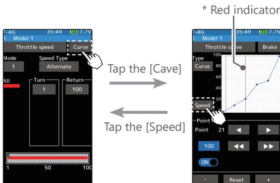
When in Alternate mode, the red indicator on the curve screen represents speed.
