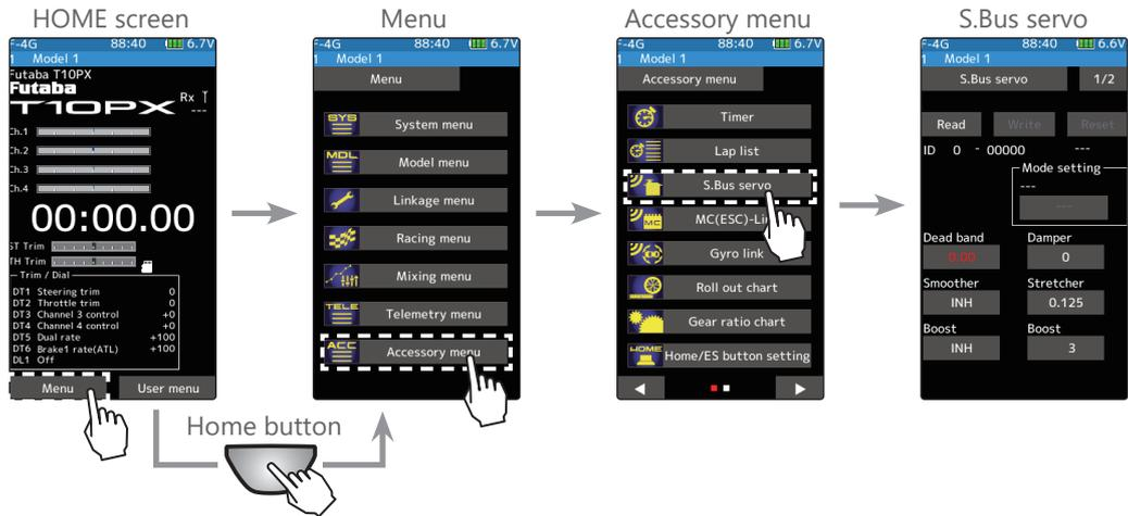
**3** Read the connected UR servo data into the T10PX.
