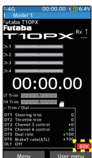
When the switch is activated, Trans-brake is visible as "BRK" on the main screen. You can now modulate the throttle and the car will not move until the Trans brake switch is released.
