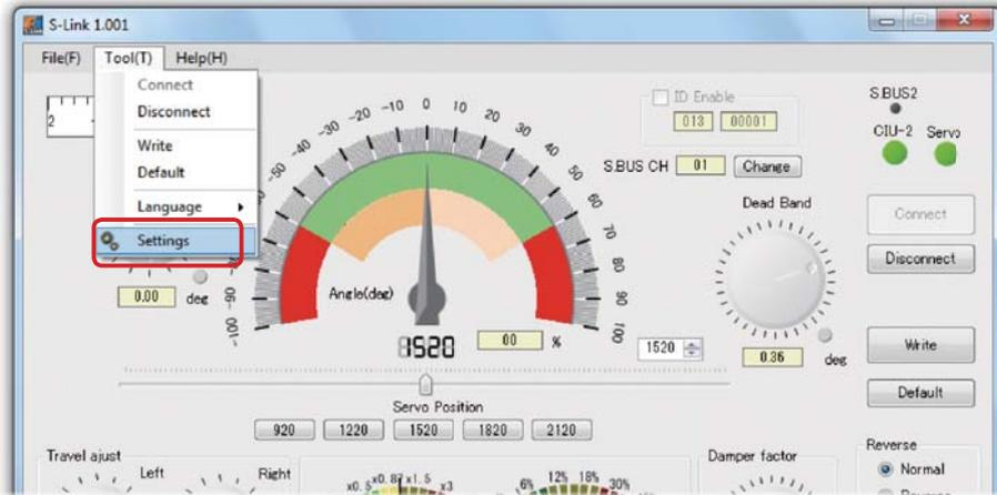
\*When the "When ending, data on display is not saved." check box is unticked before starting the parameters data at the end of the last session is displayed.
