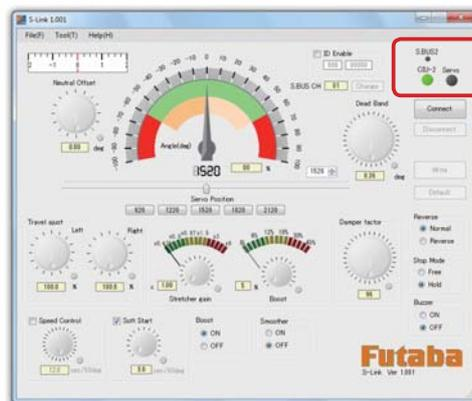
\*When the CIU-2 lamp of the screen did not light green and the following message was displayed the CIU-2/3 is not properly connected to the computer. Click "OK" and check the connection.
